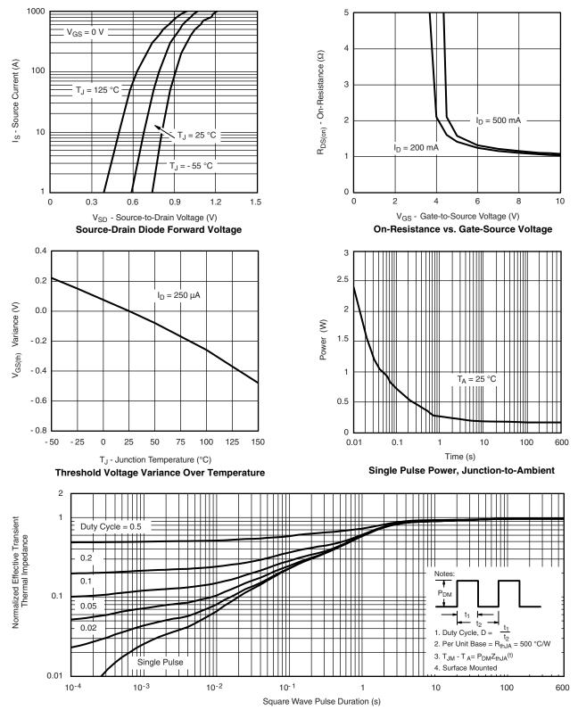
Normalized Thermal Transient Impedance, Junction-to-Ambient
